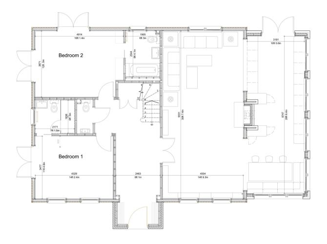
Ground Floor Plan Gross Gnd FL Internal floor area 141m'
